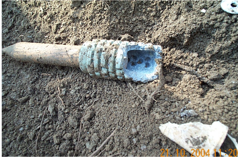
Figure 8 – Shattered remains of the PMR-2A mine
