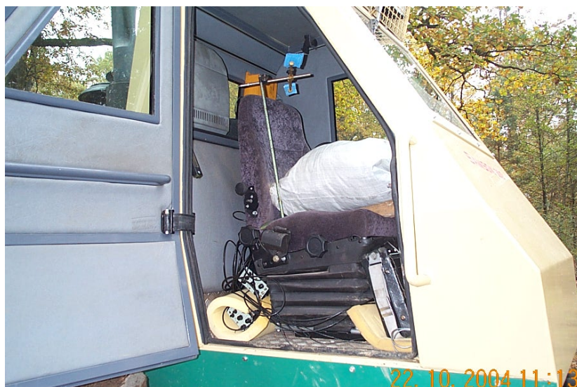
Figure 13 – Measuring instruments inside the cabin for noise and acceleration measuring in the moment of a TMA-3 mine activation
