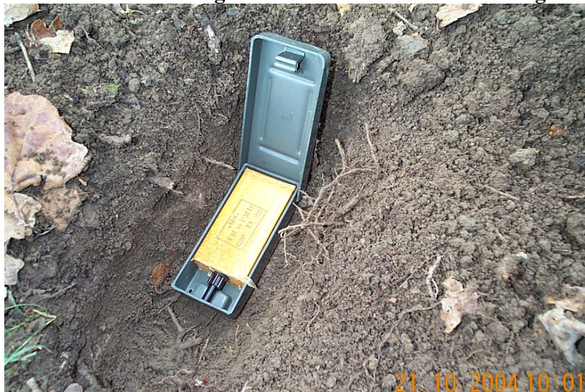
Figure 4 – PMA-1A mine prepared for testing
