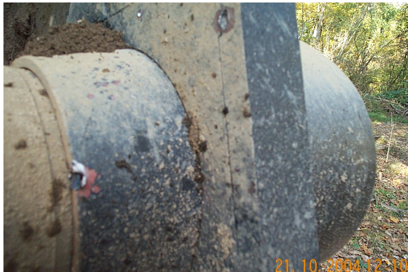
Figure 11 – Damage on the flail inflicted by the PROM-1 mine
