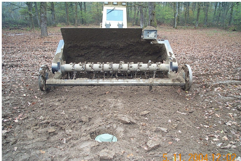
Figure 15 – TMM-1 mine prepared for testing
