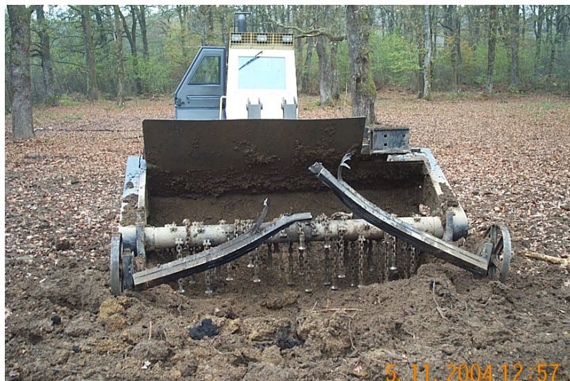
Figure 17 – Damaged vegetation rod after TMRP-6 activation
