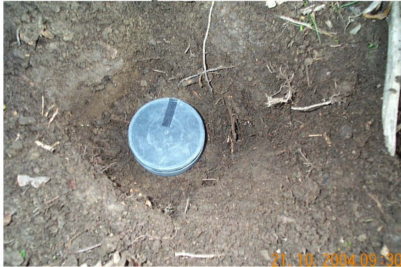
Figure 6 – PMA-3 mine prepared for testing
