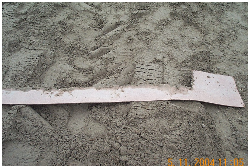
Figure 21 – Damaged fiberboard on the sand lane
