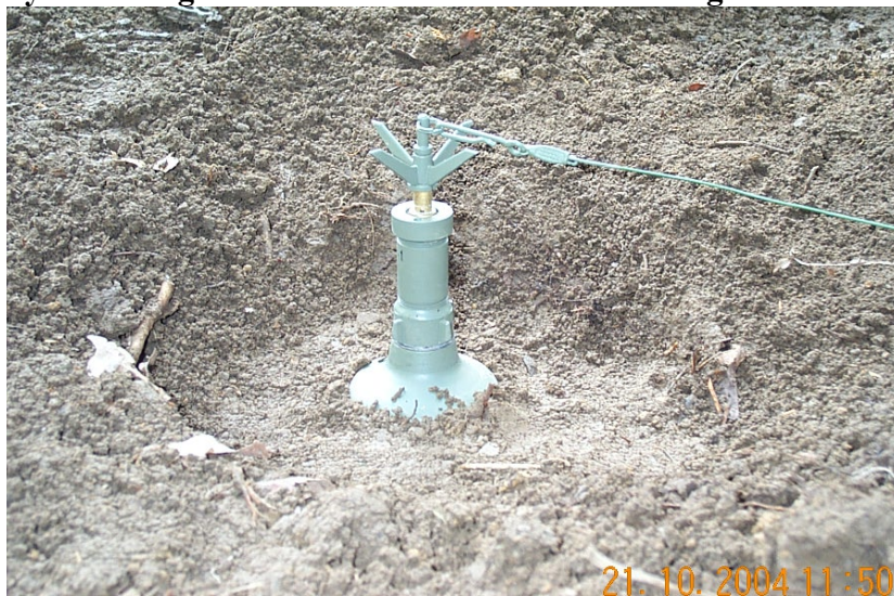
Figure 9 – PROM-1 mine prepared for testing
