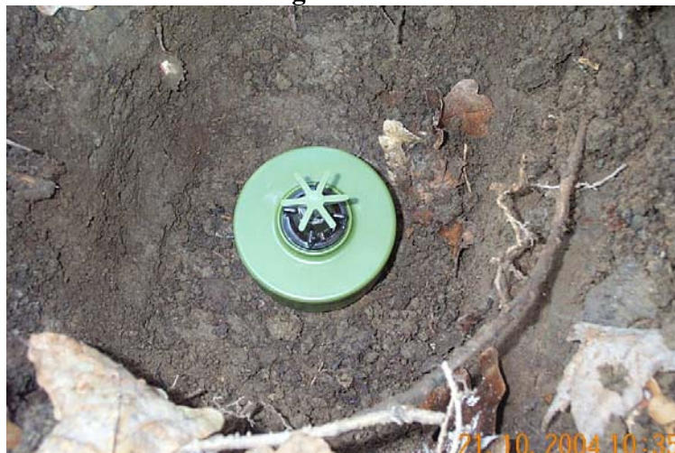
Figure 5 – PMA-2 mine prepared for testing
