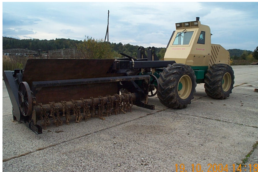
Figure 2 – „Samson 300“ demining machine prepared for transportation
