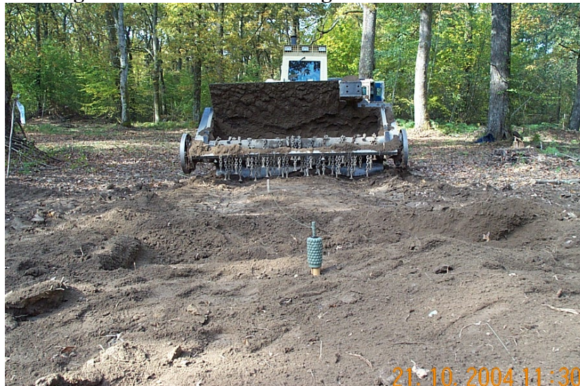
Figure 7 – Testing with PMR-2A mine
