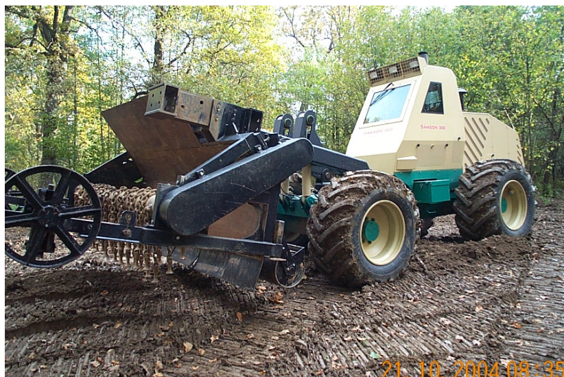
Figure 1 – „Samson 300“ demining machine
