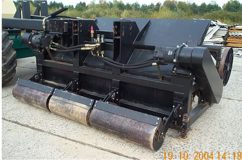
Figure 3 – The rollers on „Samson 300“ machine
