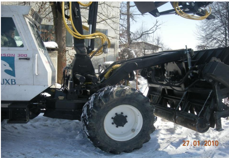
3. CHASSIS AND FLAIL UNIT WITH TILTING MECHANISM
